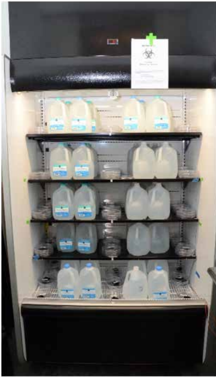
Figure 4. Commercial refrigeration unit loaded as per manufacturer's instruction using water jugs for thermal mass and stocked with inoculated powder-coated coupons
